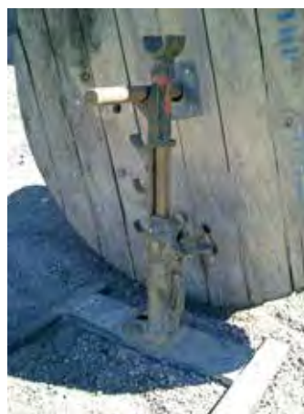
◀ Two CR321B Reel Jacks are used to support this cable spool for line feeding.
